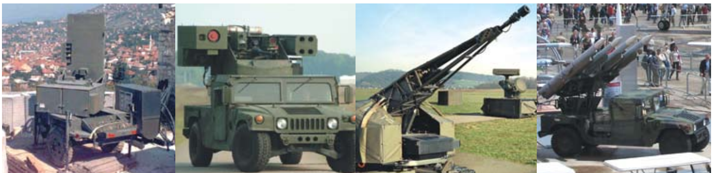
NEW SOLUTIONS FOR GBAMD THREATS: The US Army is upgrading its legacy AN/TPQ-36 target acquisition radars (far L) as a baseline to feed new ground-based air and missile defence systems capable of engaging rockets, artillery, mortars and even enemy tactical UAVs. An advanced targeting assisted laser system mounted on an 'Avenger' combat vehicle (L) offers more than GBAMD capabilities, and can neutralise IEDs and unexploded ordnance. Rheinmetall's new Air Defence Group has continued to support development of Oerlikon's 'Skyshield' C-RAM (R) which is now headed for German troops in Afghanistan, while Raytheon is offering a surface-launched version (far R) of the AMRAAM air-to-air missile already in-service with large numbers of western air forces.
