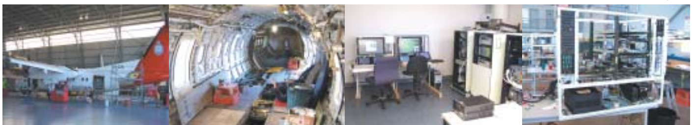
SELF RELIANCE IN MARITIME SURVEILLANCE: Adelaide-based National Air Support takes stock-standard Dash 8s (far L) and undertakes substantial modifications (L) to incorporate new digital sensors and communications equipment. To prove its CMS04 design concept and integration approach, a full test & integration laboratory was established (R), while NAS engineers also worked out a unique racking system (far R) for fitment within the luggage compartment at the back of the aircraft to accommodate all the new hardware.
